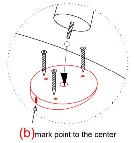
Note: Do not tighten the screws completely.
